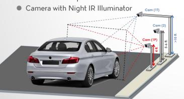
Cam 1P/1T - LPR Cam in Parking Lot Entry/Traffic Lanes, Cam 2 - Face Capture Cam\*- Optional for driver Face Image
